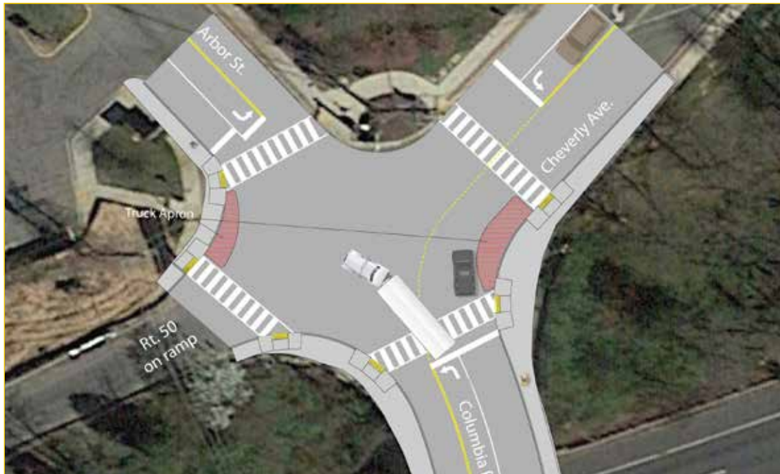
Redesigning the intersection of Columbia Park Road, Cheverly Avenue and Arbor Street can address pedestrian safety concerns leading to the Cheverly Metro station.
