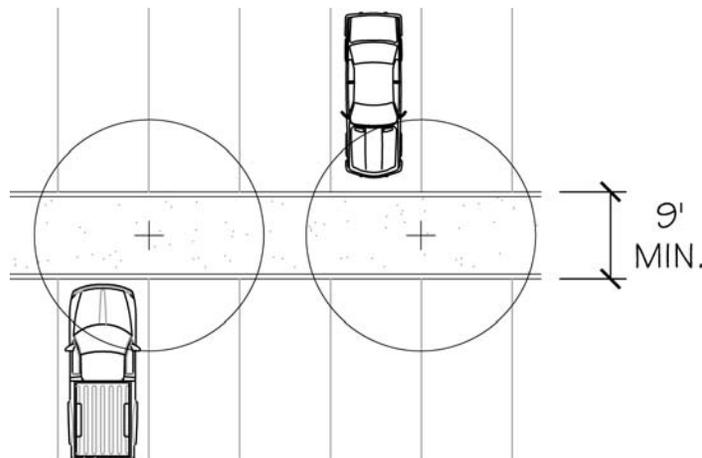
Figure 4.3-9 Minimum Width of Landscape Island Perpendicular to Spaces (parking on both sides)
