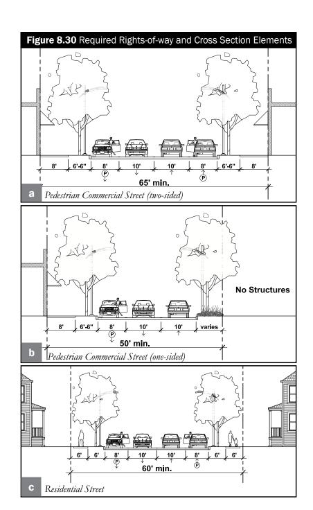
Table 8.12 summarizes the required street elements and their widths for the roadway types defined on the previous page (see Figures 8.30a through 8.30c)
