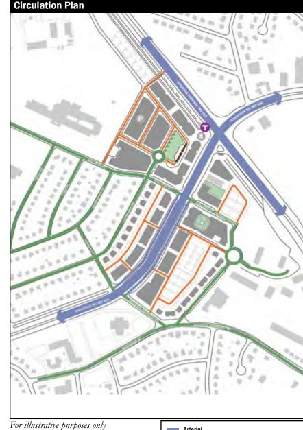
Arterial Secondary access road On-site roadways and driveways would incorporate right-turn-in/right-turn-out access to Veterans Parkway and an overpass across the future Purple Line right-of-way.
