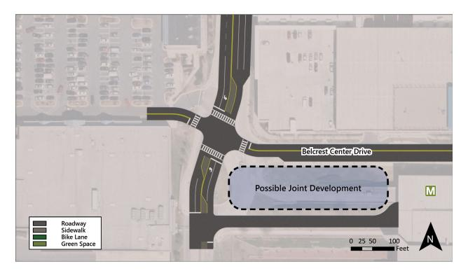
Figure 34. Belcrest Center Drive, reconfiguration of teardrop to four-way stop
